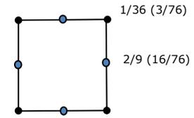
QUAD8 HRZ lumped mass ratio based on 2x2 integral vs. 3x3 integral (in parenthesis)
