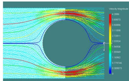
The 3D version of the CFD benchmark compares the mass conservation of a moving ball in the channel flow problem. Automatic meshing with an average mesh size of 0.07 is used for all mesh types. Half symmetry is used.
