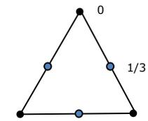
TRI6 HRZ lumped mass ratio based on 4-point integral
