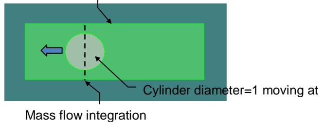
The mass conservation error at the narrowest flow section is computed by integrating the total flow passing the cross section plane. Automatic meshing with an average mesh size of 0.04 is used for all types of meshes.
