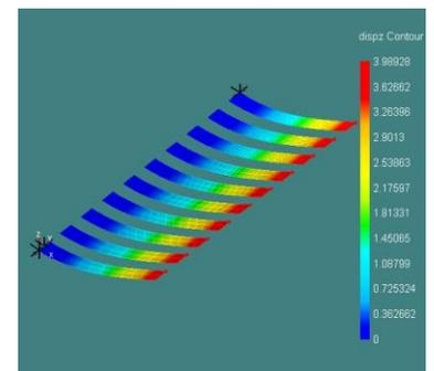
Two types of patch tests have been performed. The first patch test applies a fixed deformation to check the uniform strain field, and the second test uses an external uniform pressure loading to test the stress variation. A minimum of one completely constraint free element is included in the domain, and both 2D and 3D domains are tested using Sefea low order element formulation. In both cases, both 2D triangle Sefea TRI3 and 3D Sefea TET4 show uniform strain and stress perfectly.
