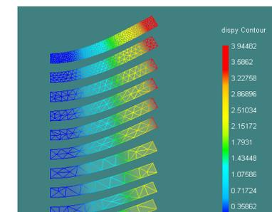
Similar to the 3D benchmark, ten 2D plane-stress cantilever beams of size 1x10, Young's modulus=1000, Poisson's ratio=0.35 with a free-end distributed shear load=1 are used to demonstrate the Sefea 2D behavior. Each beam is meshed with an average triangle mesh size from 2 to 0.2, with increment of 0.2. The mesh variations and sizes are even coarser than the 3D case and are usually not recommended, except for the demonstration of theoretical benchmarks.
