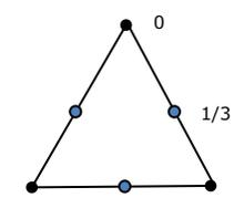
TRI6 HRZ lumped mass ratio based on 4-point integral
