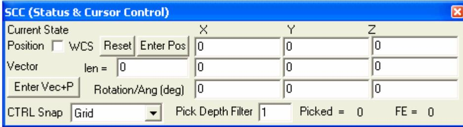
6. You can move the mouse onto the screen to verify that you have entered a point at the global origin (0, 0, 0). The global origin is displayed on the screen as three small axes lines that match the axes color of the orientation axis at the bottom right of the screen.
